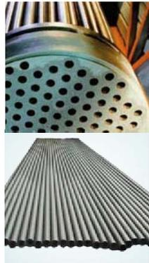
OUR GRAPHITE TUBES ARE MANUFACTURED IN FRANCE BY AN EXTRUSION PROCESS WHICH PRODUCES UP TO 6 METER LONG TUBES WITHOUT A JOINT. THE TUBES HAVE THE HIGHEST MECHANICAL RESISTANCE (G30-00-220) CERTIFIED BY TÜV. THE GRAPHITE SHELL AND TUBE HEAT EXCHANGERS CAN BE ASSEMBLED IN ALL OUR WORLDWIDE WORKSHOPS.
